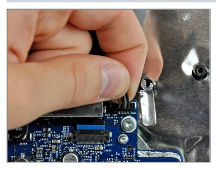
Lift the optical drive fan connector straight up out of its socket on the logic board.
