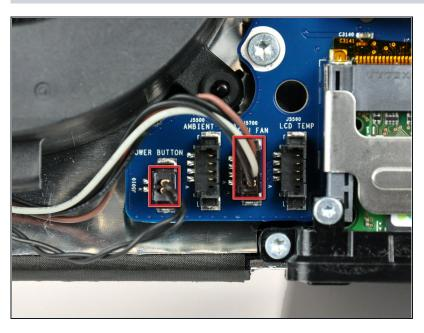
Disconnect the power button and CPU fan by lifting their connectors straight up off the logic board.
