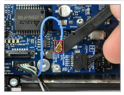
Use the flat end of a spudger to pry the Bluetooth antenna connector up off the Bluetooth board.
