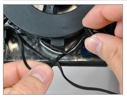
If necessary, de-route the ambient temperature sensor cable from under the power button cables.
