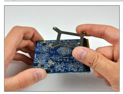
• Lift the metal heat sink bracket off the video card.
