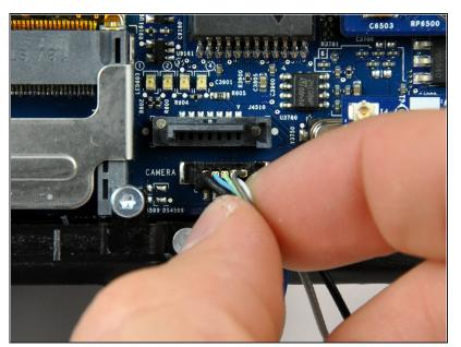
Pull the camera cable connector straight up out of its socket on the logic board.
