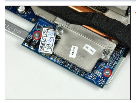
Remove the two 5 mm T8 Torx screws securing the video card to the framework on the logic board.
