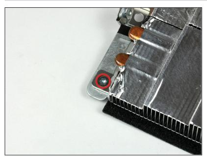
Remove the 4.3 mm T8 Torx screw securing the video card heat sink to the framework attached to the logic board.
