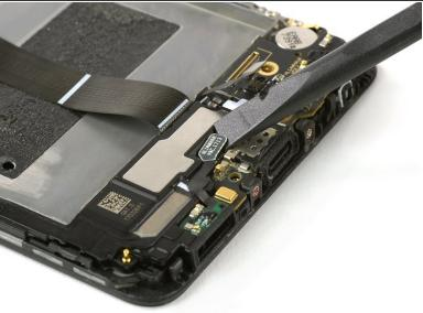
Use a spudger to disconnect the loudspeaker and the charging port flex cable from the daughterboard.
