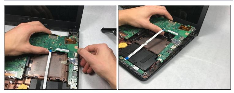
• Grip the motherboard firmly and pull the board leftward and upwards so that the ports on the right side escape their frames.
