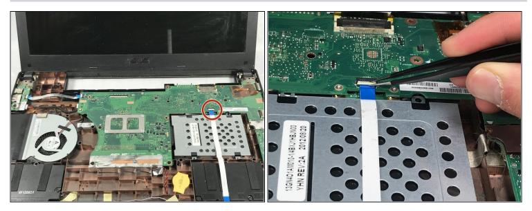
• Unlatch the data cable by using <u>tweezers</u> to lift the white tab and release the cable.
