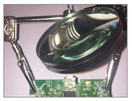
Prepare your station for the desoldering of the charging port.
