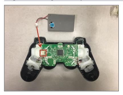
Remove battery by unlatching the battery cables from battery connector clip.
