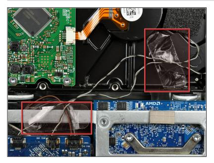
If necessary, remove the pieces of tape securing the hard drive/optical drive thermal sensor cables to your iMac.
