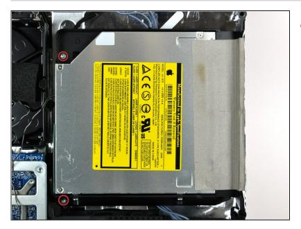
Remove the two fine-thread 7 mm T10 Torx screws securing the optical drive to the rear case.
