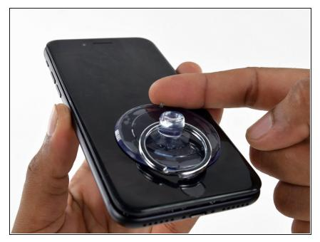
• Lift the small appendage of the suction cup to remove the instrument from the front panel.
