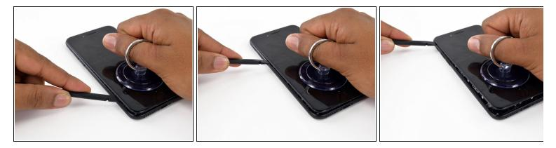
• Slide the spudger along the left side of the iPhone, starting at the bottom and moving to the volume control buttons and the silent mode switch.
