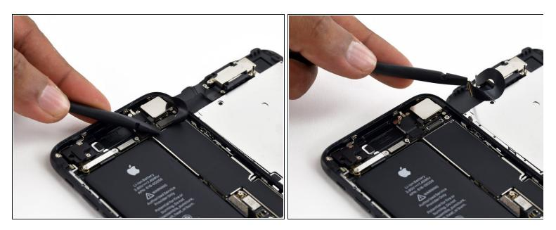
• Disconnect the front panel sensor assembly connector from its socket on the logic board.
