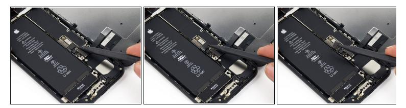
• Use the pointed end of a spudger to lift the battery connector from its socket on the logic board.
