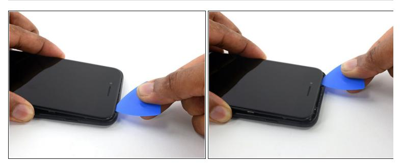
Slide an opening tool along the top side of the iPhone, between the back case and the front panel, to break the rest of the sticker that holds the screen in place.
