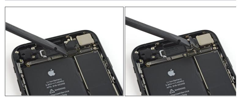
Use the flat end of a spudger to disconnect the rear-facing camera's press connector from its socket on the logic board.
