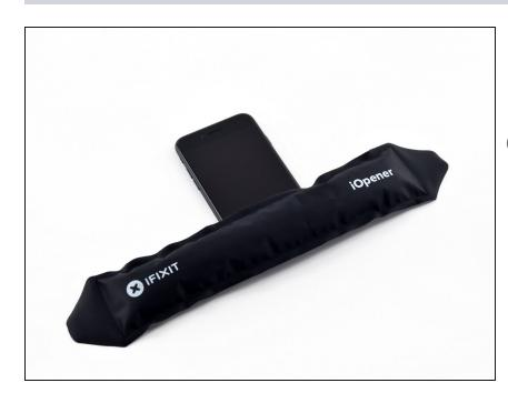
• Put the hot iOpener over the bottom of the phone to soften the adhesive that holds the display.
