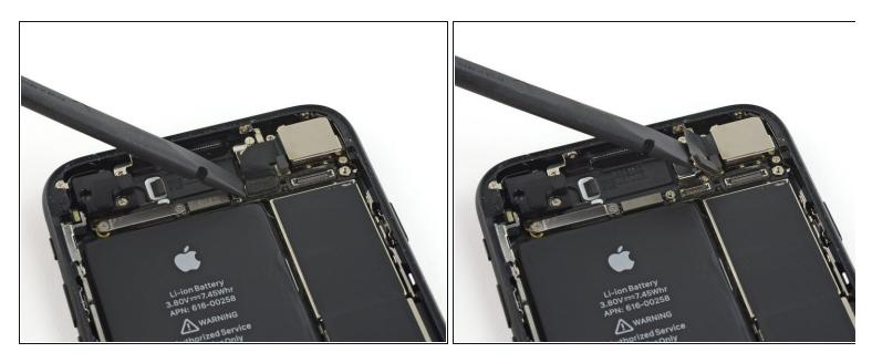
• Use the flat end of a spudger to detach the rear camera's pressure connector from its seat on the logic board.
