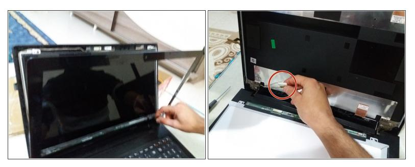
Remove the cable from the old screen and install it in the new screen in the same way.
