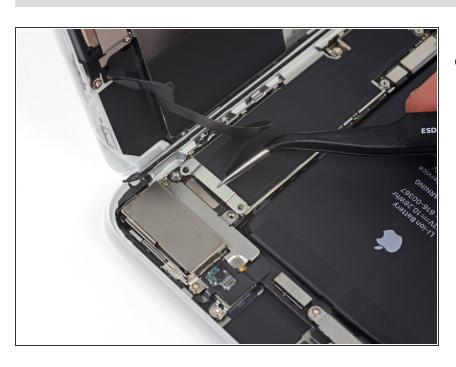
Remove the bracket covering the front panel sensor assembly connector.
