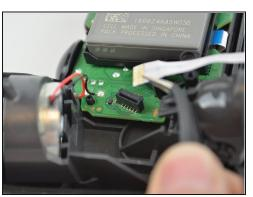
Pull the ribbon cable out of the motherboard port to fully separate the two halves, using a pair of <u>tweezers</u>.
