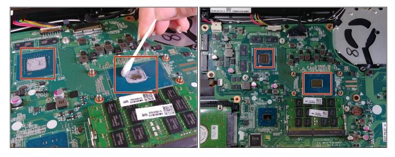
• Repeat the same cleaning process from the previous step on the matching thermal plates on the motherboard.
