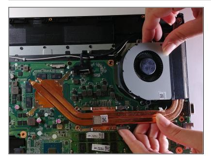
• Gently re-seat your component, making sure that the thermal plates align correctly.
