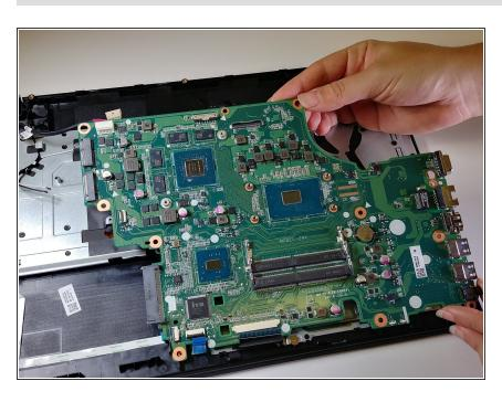
Lift the motherboard gently to completely remove this component from the device.
