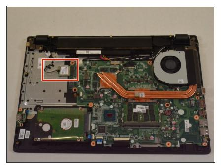
Locate the wireless card on the top left quadrant. It should have two antenna cables connected to it, one white and one black.
