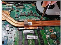
Use a Phillips #1 screwdriver to remove 6 black 10mm Phillips Head screws that connect the copper heat-sink to the motherboard.
