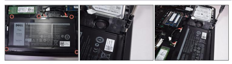
• Unscrew the 5 x 2mm x 5mm screws, using the T8 Torx screwdriver.
