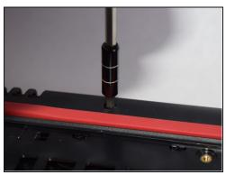
• Using the Philips #1 screwdriver, unscrew the 4 x 2mm x 5mm screws, located on the top of the laptop.
