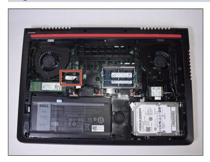
Locate the LCD cable, near the center of the laptop.
