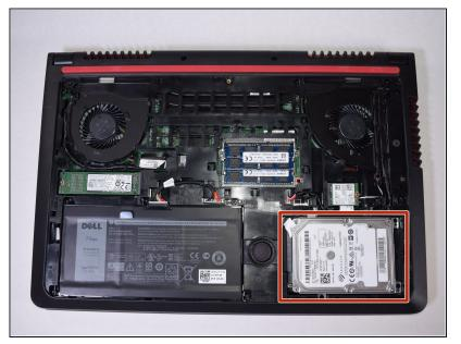
• Locate the hard drive on the bottom right side of the laptop.
