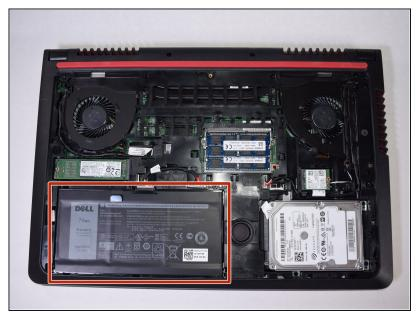
• Locate the battery on the bottom left side of the laptop.
