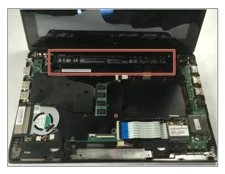
The battery will be easily visible towards to top of the internals. It is a long, black rectangle marked "Liion". Notice that the battery is currently secured by three screws. We will need to unscrew them in order to remove the battery.
