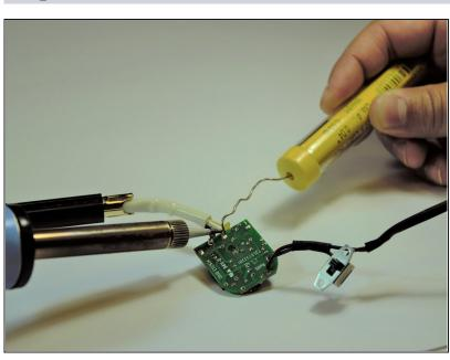
To reattach the new temperature control switch, solder the piece onto the board.
