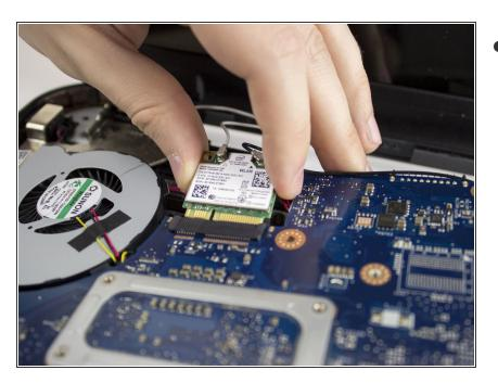
Remove the Wi-Fi chip by pulling upwards.
