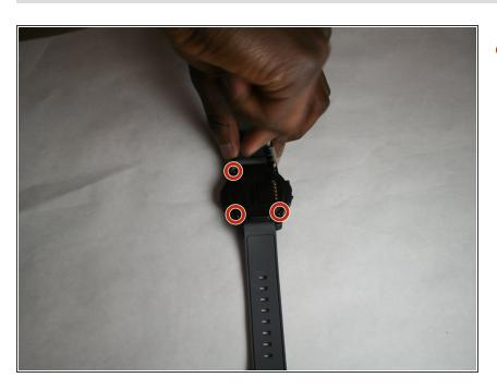
Unscrew 4 4.5mm Phillips head screws from the back of the device.
