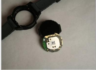
Separate motherboard from screen and then clean or replace motherboard.
