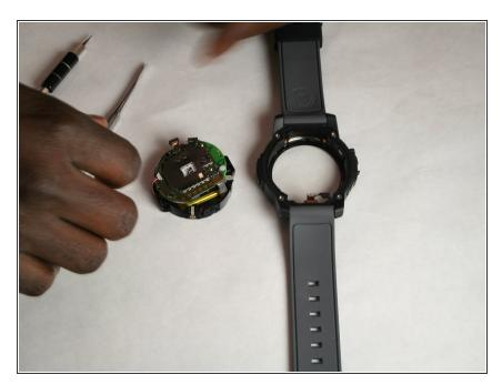
Remove the "core" of the device from case.
