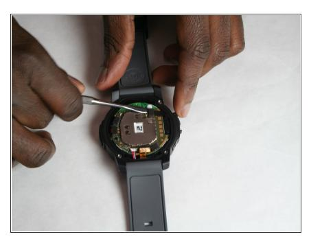
Unclip straps holding motherboard to screen using a spudger.
