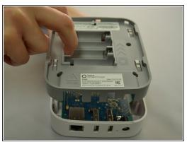
Once all five screws are removed, split the casing apart by applying gentle upwards pressure against the positive terminals in the battery compartment.
