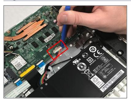
Using a plastic opening tool, disconnect the wires connecting the battery to the motherboard.
