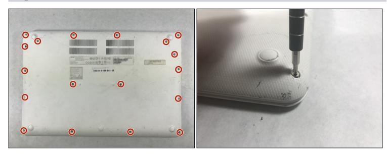
Remove the following eighteen screws using a Phillips #0 screwdriver.
