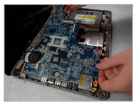
Lift up the right side of the motherboard and pull it out to the right carefully.
