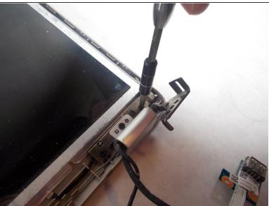
After the bezel is removed you have to remove the 6 screws on the bottom corners and two that are located on the top corner with a Phillips #1 screwdriver.
