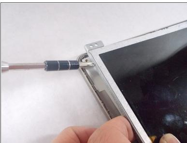
Then you with a Phillips #1 screwdriver must remove the 4 screws that are on the edges of the screen, which are holding the screen to the screen brackets. There are 2 on each edge.
