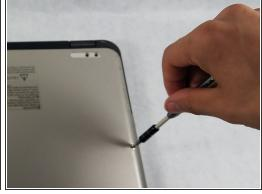
Remove the ten 5mm Phillips #0 screws that secure the back plate to the computer.
