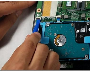
Use a plastic opening tool to detach the hard drive's ribbon cable from the computer. Gently lift the black lever at cable's point of attachment to the computer to release it.
