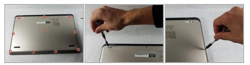
• Remove the ten 5mm Phillips #0 screws that secure the back plate to the computer.
