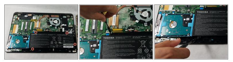
Remove the four 3mm Phillips #0 screws connecting the battery to the computer.
