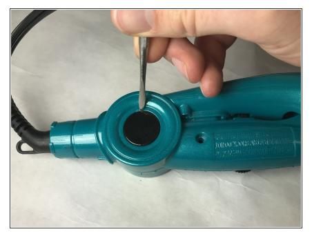
Pry the black screw cover off the side of the lower handle housing using a fine-point spudger or pick. This side will have the model number and other product information embossed on it.
