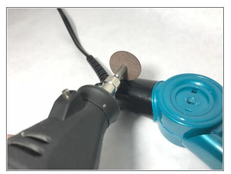
• Cut along the length of the black housing retainer with a rotary tool to split and remove the retainer.
