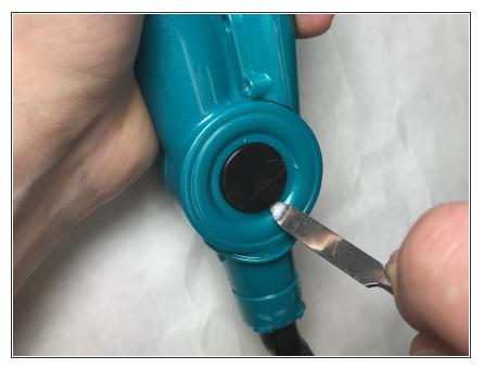
Pry the black screw cover off the other side of the lower handle housing. This side will have the power switch located on it.
