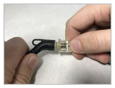
• Gently pull the power cord out of the power lead connector.
