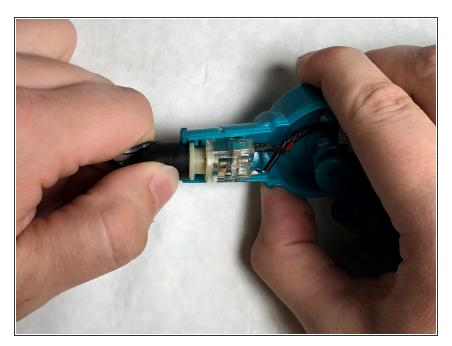
Pull upward on the power cord connector to remove it from the lower handle housing.
