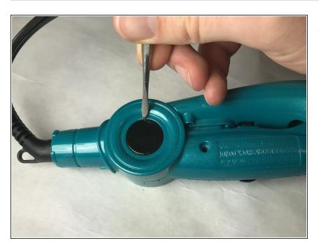
Pry the black screw cover off the side of the lower handle housing using a fine-point spudger or pick.
