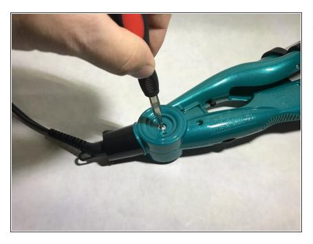
Remove one 10 mm Phillips 1 screw from the handle joint.
