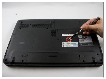
Remove the (mm) screw in between the two white manufacturer's stickers using the Phillips #1 screwdriver.
