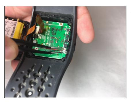
Use some tweezers to remove the small white clip for the battery from the circuit board.
