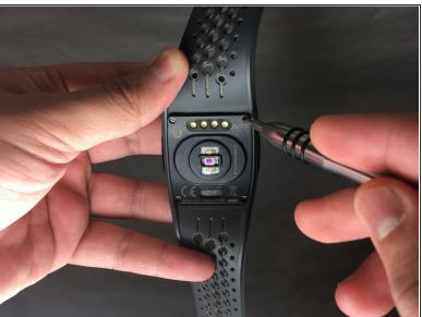
Remove the 4 JIS 00 6.71 mm screws.
