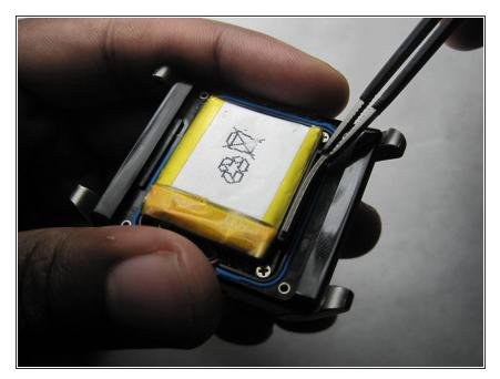
• Use tweezers to remove elastomeric, or zebra, connector.
