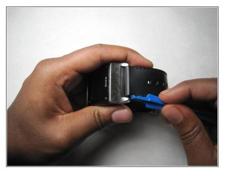
• Wedge a plastic opening tool between band contacts.
