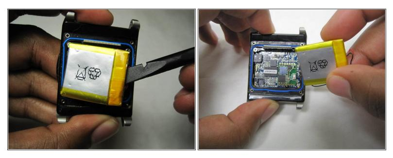
• Use the flat end of the spudger to carefully lift the battery until adhesive seal is broken.
