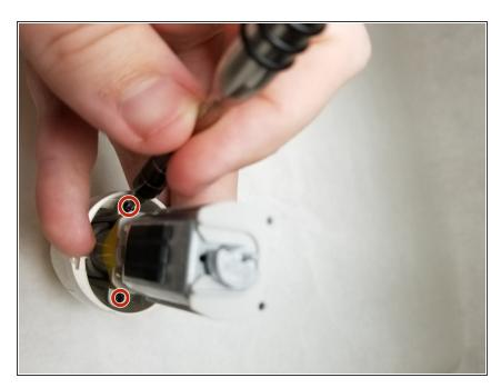
Remove (2) 7.9mm Phillips #0 screws and remove endcap from frame.
