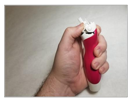
Push the blade mount assembly towards the rear of razor and remove.
