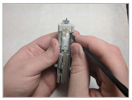
Using pointed end of spudger, push on the motor through the hole in the back
