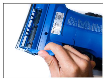
Pry off the Riser Visor using the plastic opening tool.
