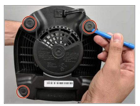
Use the prying tools to open the four plastic screw holes on the bottom of the blender.
