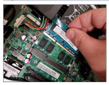
Carefully slide the RAM card out of its slot, and insert the replacement card
