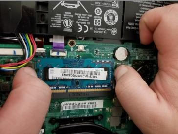
• Locate the RAM slot and push outwards on the metal tabs to release the RAM card.
