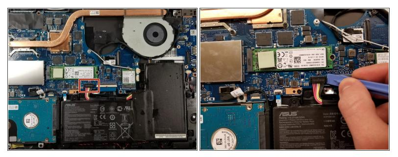
• Wedge an opening tool under the battery's bundled cable connector, and gently pry the connector up and to disconnect the battery.
