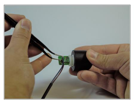
Desolder the two connected electrical wires. Take note of the orientation of each wire to properly reassemble the device.
