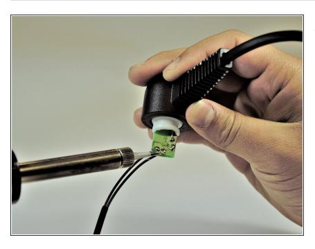
With the two electrical wires in the correct orientation, solder the wires to the new Hot Tools Professional 1110 power cord.
