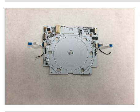
Separate the motherboard from both LED chips.
