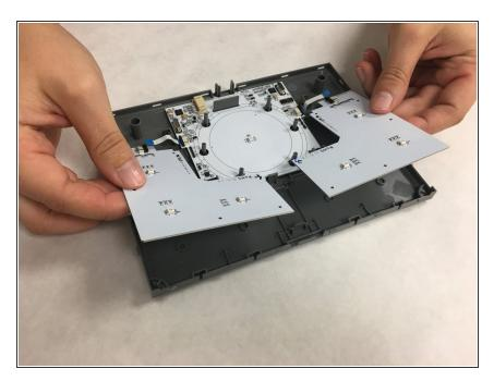
Lift up both LED chips. As you are lifting, pull towards the motherboard to release it from the toy pad cover.
