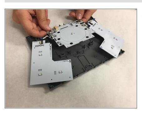
Lift up the motherboard, and remove the motherboard and LED chips from the toy pad.
