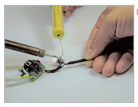
Ensuring that the three connecting electrical wires are in the correct orientation, solder the new power switch to the wires.
