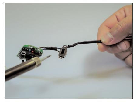
Remove power switch from the housing and desolder the three connected electrical wires. Take note of the orientation of each of the electrical wires to ensure that they are replaced correctly.
