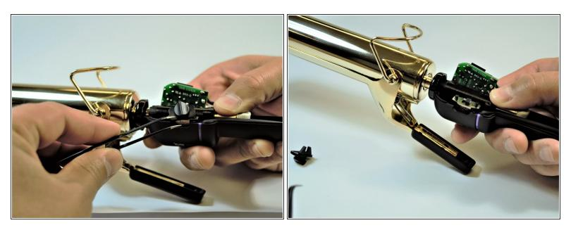
• Remove the power switch button exposing the electrically connected power switch.
