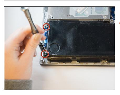
Remove the two 4.4mm Phillips#00 screws from the battery case.
