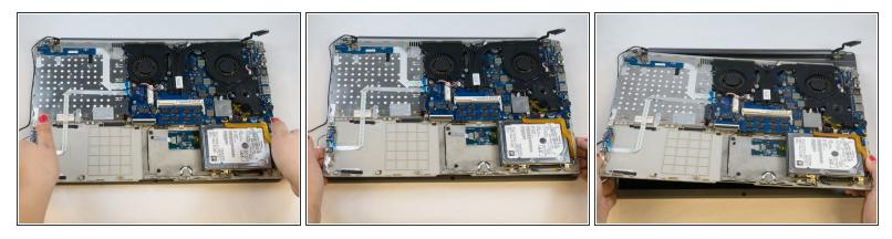
Using your fingers, grasp the edges of the inner case then lift and pull away to separate it from the display.
