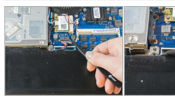
Using tweezers or your fingertips, carefully pull on the battery connector to disconnect it from the motherboard.
