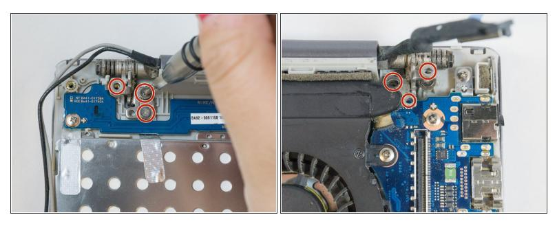
Using the Phillips#00, remove the six 4.5mm screws from the corner brackets holding the display to the inner case.
