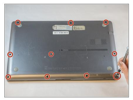
Remove the ten 6.6mm Philips#00 screws securing the lower case to the upper case.
