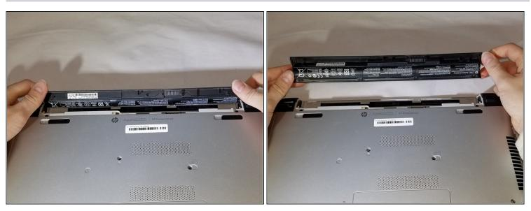
Lift the battery upwards and out from the laptop
