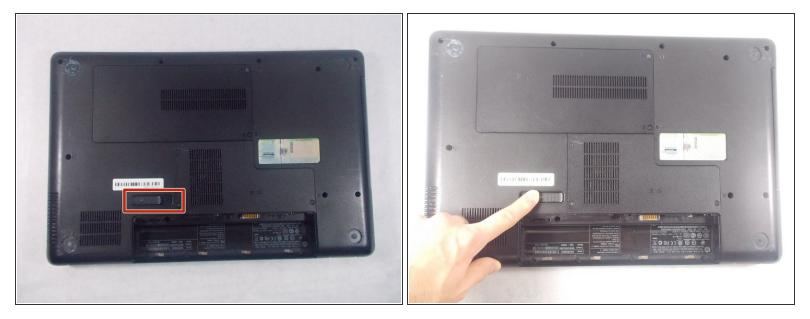
$\bigwedge$  Make sure to turn off the laptop before removing the battery.
