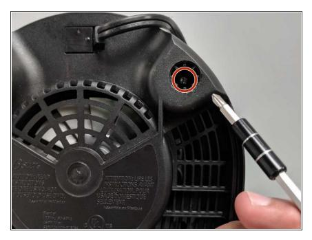
Use the Phillips #1 Screwdriver to unscrew the four 16 mm screws and remove the plastic bottom.
