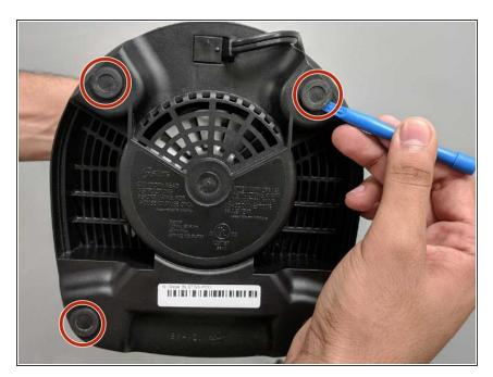
Use the prying tools to open the four plastic screw holes on the bottom of the blender.
