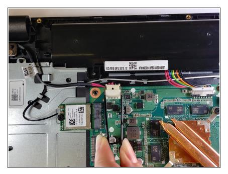
With a pair of blunt tweezers, push on the side tabs of the connector to disconnect the harness from the motherboard.
