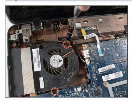
• Remove the two screws securing the fan using the Phillips #1 screwdriver .
