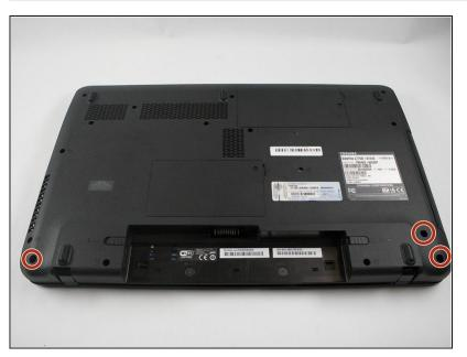
Remove the three screws from the underside of the laptop using a Phillips #1 screwdriver.
