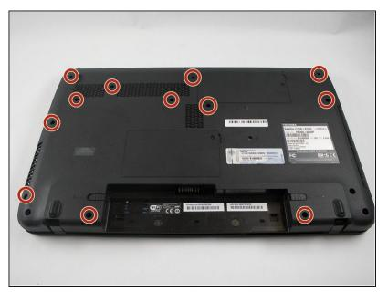
Remove the twelve screws from the underside of the laptop using the Philips #1 screwdriver.
