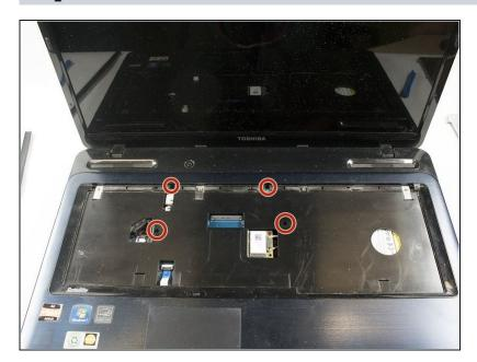
Remove the four screws securing the keyboard using the Philips #1 screwdriver .
