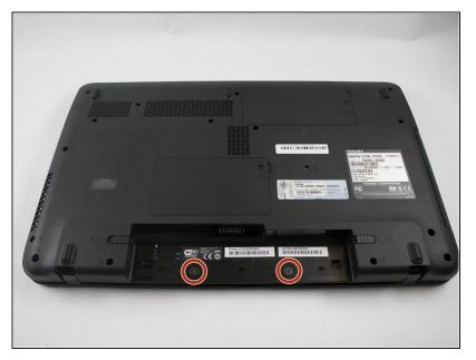
Remove the two screws from the underside of the laptop where the battery was located using the Philips #1 screwdriver.
