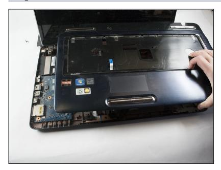
Remove the top plastic cover by lifting from one of the corners it should be easy to removed.
