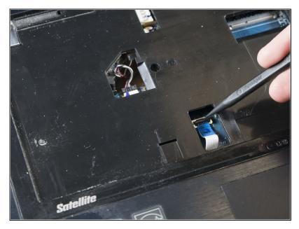
Detach the ribbon cable carefully using the spudger to gently pry up on the clip until it releases the ribbon cable or lift up on the blue tab gently until the clip releases the ribbon cable.
