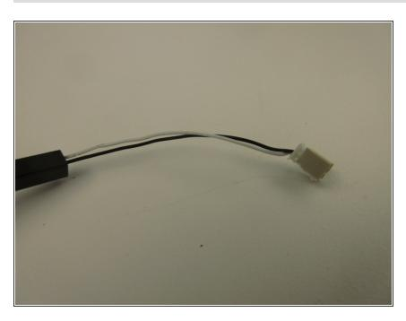
Cut the connection head off and pull the wiring out of the leg. To reassemble your device, follow these instructions in reverse order.
