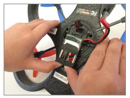
• Push the battery upward with your thumbs to loosen it from the tight slot until your thumbs can not reach the bottom of the battery anymore.
