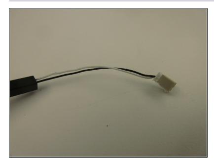
• Cut the connection head off and pull the wiring out of the leg.
