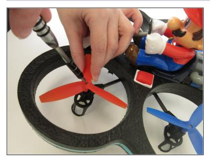
• Using the JIS #00 screwdriver, hold the rotor blade still and unscrew the 4.762mm screw in the center of the blade.
