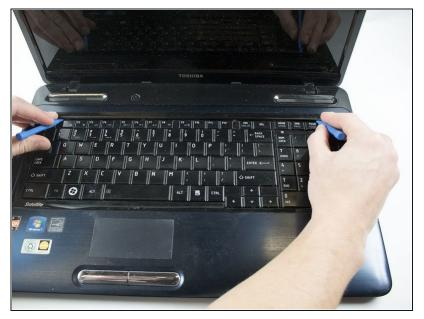
Pry up the thin narrow strip of facing above the keyboard using the opening tool.
