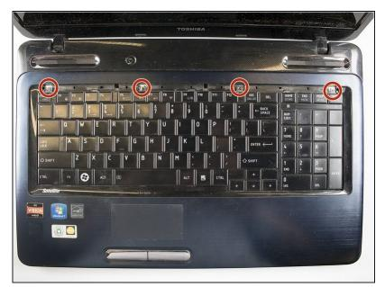
Remove the four screws securing the keyboard using the T4 Torx screwdriver,
