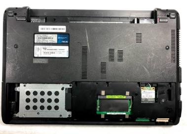
Slide the back panel off by placing a hand on each corner and pulling the panel towards you.
