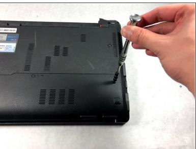
Use a Phillips #000 screwdriver to remove the two 9mm screws from the HDD/RAM cover panel.
