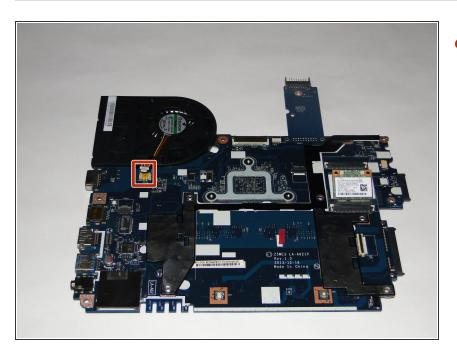
Detach the connector between the fan and the motherboard.
