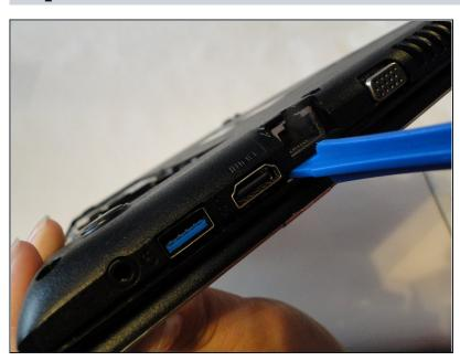
Using a plastic opening tool, carefully separate the frame along the edges of the laptop.
