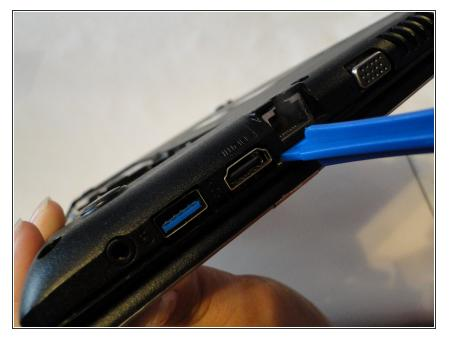
Using a plastic opening tool, carefully separate the frame along the edges of the laptop. This should separate the keyboard assembly from the bottom portion of the laptop.
