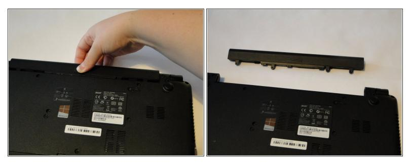
• Carefully slide the battery out of the battery's home.
