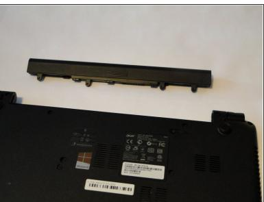
Carefully slide the battery out of the battery's home.
