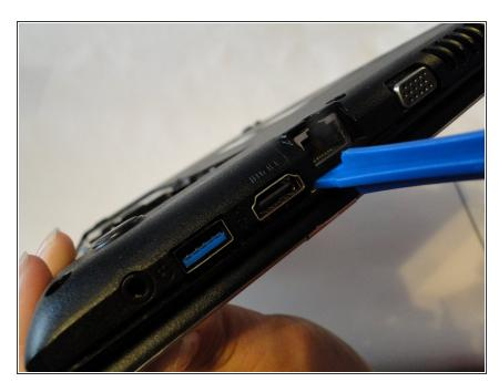
Using a plastic opening tool, carefully separate the frame along the edges of the laptop. This should separate the keyboard assembly from the bottom portion of the laptop.
