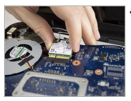
Remove the Wi-Fi chip by pulling upwards.
